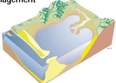
**Figure 1.** A 3-D geomorphic conceptual model of a wave-dominated estuary
