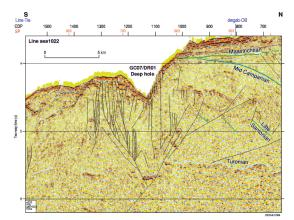
Figure 3. AUSTREA-1 seismic reflection profile across a 240metre-deep hole in the Nullarbor Canyon. The shape of the hole is controlled by deep faults taking root at the base of the Turonian shaly unit. The shales form a décollement for younger growth faults along which water escapes when the shales are over-pressured.
