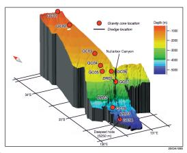
Figure 2. Seafloor topography and canyon systems of the Great Australian Bight Marine Park, produced from AUSTREA-1 swath data. The view is to the north-east and shows an area about 130 kilometres long. The location of AGSO samples acquired during the Southern Surveyor cruise is indicated by red circles for the cores and by black lines for dredges.
