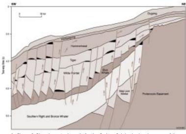
▶ Figure 2. Play element schematic for the Ceduna Sub-basin showing some of the main sequence stratigraphic subdivisions within the Bight, structural elements, and various numbered play types within the basin.
