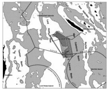
Figure 2. Map of a large part of the Fairway Basin, showing the distribution of the largest 'salt' domes and ridges, and of the 'bottom simulating reflector' representing gas hydrates, in relation to water depth.
