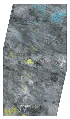
▲ Figure 4. Combined phengite (yellow) and muscovite (blue) mineral maps draped over grey-scale 1 ASTER image. Individual index maps were clipped using a mean plus two standard deviation algorithm, then recoloured. Phengite forms a broad zone to the south whereas muscovite is restricted to the north. Telfer is located where the white mica changes from phengite to muscovite.
