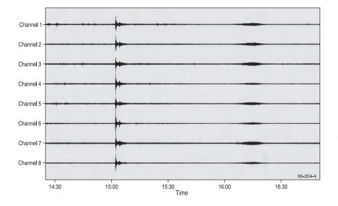
▲ Figure 4. Macquarie Ridge magnitude 8.1 earthquake signal recorded on the IS05 infrasound station. The earliest arrival is the P phase, followed by S, and some time later by the airborne acoustic signal.
