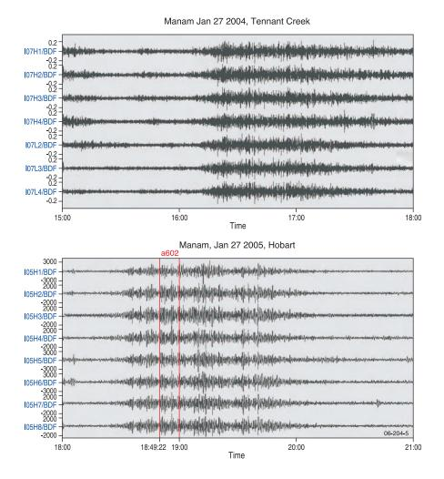
▲ Figure 5. Acoustic signals from the eruption of Manam volcano of 27 January 2005, recorded on (a) IS07, filtered between 0.4 and 1.6 Hz, and (b) IS05, filtered between 0.03 and 0.1 Hz.
