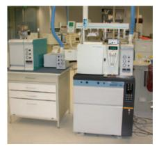
Gas chromatography – stable isotope mass spectrometer used in hydrocarbon isotope analysis.
