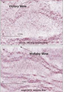
**Figure 3.** Seismic reflection lines (3A, 3B) across the Victory and Wallaby gold deposits showing both located above the apex of domes. The muted regions between the strong reflectivity is interpreted as a granite laccolith. The diffuse zone cross cutting the strong reflectivity at the Victory gold mine (3A) is mapping swarms of porphyry dykes that are likely sourced from the laccolith (dome) at depth.
