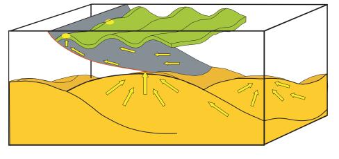
▲ Figure 2. Schematic model (from Henson et al 2005) of fluid focusing towards mineral deposits (yellow dots) above a series of stacked domes with decreasing wavelengths (black horizontal lines) upwards.
