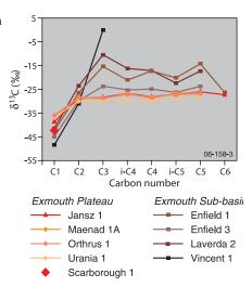
▲ Figure 4. Carbon isotopic values for individual gas components from the Exmouth Sub-basin, emphasising the effects of biodegradation.
