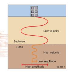
▲ Figure 1. Sediments near the Earth's surface can amplify earthquake energy waves by reducing their velocity and increasing their amplitude.
