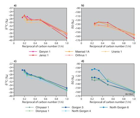
▲ **Figure 2**. Carbon and hydrogen isotopic values for individual gas components from the Exmouth Plateau and Gorgon area, highlighting source differences.
