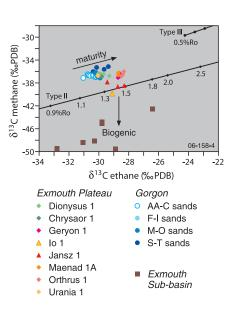
Figure 3. Plot of δ<sup>13</sup>C ethane versus δ<sup>13</sup>C methane showing kerogen type and maturity trends for the Exmouth Plateau and Rankin Platform gases, and the effect of biodegradation on gases from the Exmouth Sub-basin.
