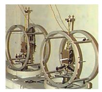
Figure 2. Gnangara's recording vault, showing the historic Eschenhagen equipment. The Eschenhagen variometer was first installed at Watheroo observatory by the Department of Terrestrial Magnetism in 1919. It was transferred to Gnangara in 1960 and operated there until 1991. This historic equipment is now on display in the Geoscience Australia building foyer.
