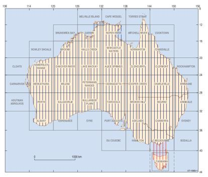
**Figure 1.** Proposed flight-line pattern for the AWAGS 2 magnetics and radiometrics survey to back-calibrate the National Radiometric Database.
