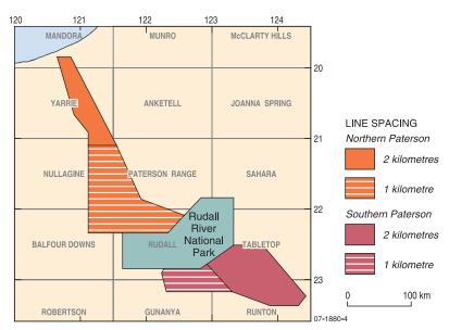
Figure 4. Proposed airborne electromagnetic survey area, Paterson Province, Western Australia.
